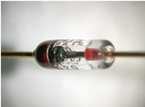
Figure 1: Closeup of a diode, showing the square shaped semiconductor crystal
